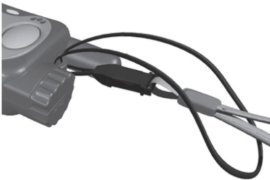
The image above shows the method of attaching the lanyard to the Pendant. Note that the lanyard has a break-away feature to release if it gets caught on something while around someone’s neck.
