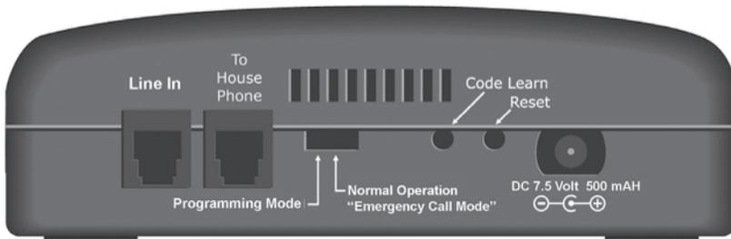
**Power Connection.** Simply plug in the AC Adapter in to the nearest electrical outlet. Plug the other end of the AC power adapter into the Base unit. You need to push the plug into the opening in the Base unit and twist 90° clockwise to lock in place. To remove in the future, simply rotate 90° counter-clockwise and pull outward.
